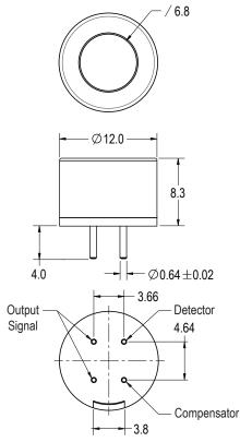
(The two signal output terminals need to be short-circuitd in actual application)
